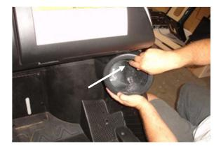
Align the speaker panel in the upper side corner of the footwell and mark the 2 holes
