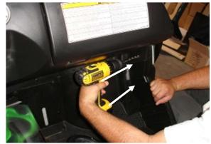
After marking the holes, drill them using a 1/4" drill bit
