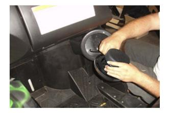
After securing all the allen bolts and the 7/16 nuts run your speaker wire into the speaker pod and attach wire to speaker
