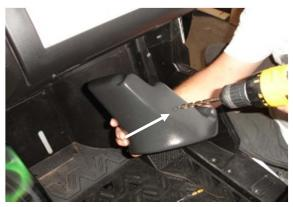
Drill a hole through the top of the pod for your speaker wire
