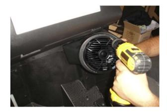
After attaching the speaker wires to the speaker install the speaker into the Wet Sounds kick panel.
